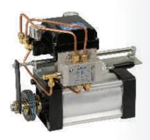
Linear cylinder with volume Booster valve for operating damper/ globe/ gate valve with positioner 4-20 mA or 5-15 psi
